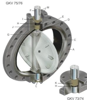
**BLOW-OUT PROOF STEM:** A retaining ring, installed between the machined stem groove and gland retainer step, provides full retention of the stem in the unlikely event of internal stem failure.
